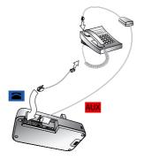
Figure 27: Connecting using an electronic-hookswitch adapter (Jabra LINK series)
